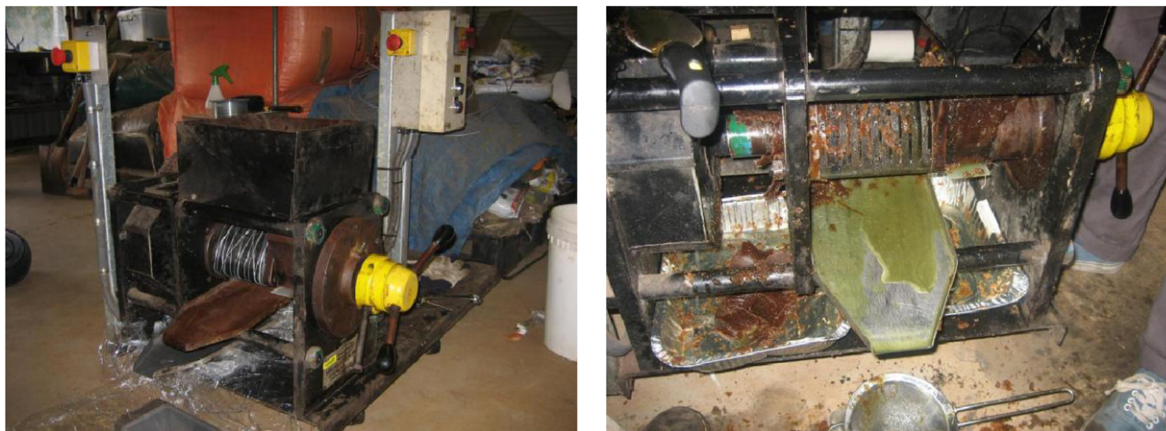
Fig. 2. Beauty leaf oil extraction using a screw press.
