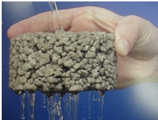
Figure 3: No-Fines Concrete (Ghafoori and Dutta, 1995)
