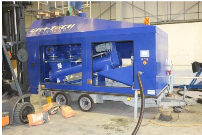
Figure 6: the GEM-TECH machine for mixing the material
