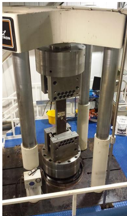
366 Figure 12. Experimental configuration of large scale dog-bone tests
