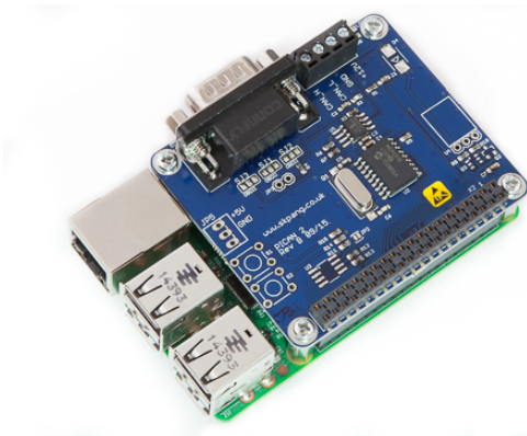
Fig. 5. PiCAN2 board 2 (blue) connected to a Raspberry-Pi (green). PiCAN2 board extends the Raspberry Pi with CAN-Bus communication ability. Connections to physical CAN bus from the PiCAN2 are enabled via a DB9 socket or a screw terminal.
