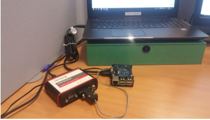
Fig. 9. The physical setup for security testing. CANoe and the virtual ECUs run on the laptop. The QRNG ECU (Raspberry and PiCAN2), in the middle, is connected to the laptop via the VN1630 box (coloured red, white and black).
