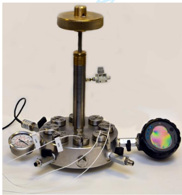
Fig. 4 Saturation chamber: (a) schematic diagram; (b) photo
