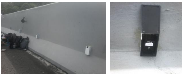
Fig. 7 Bridge vibration data collection using SunSPOT node
