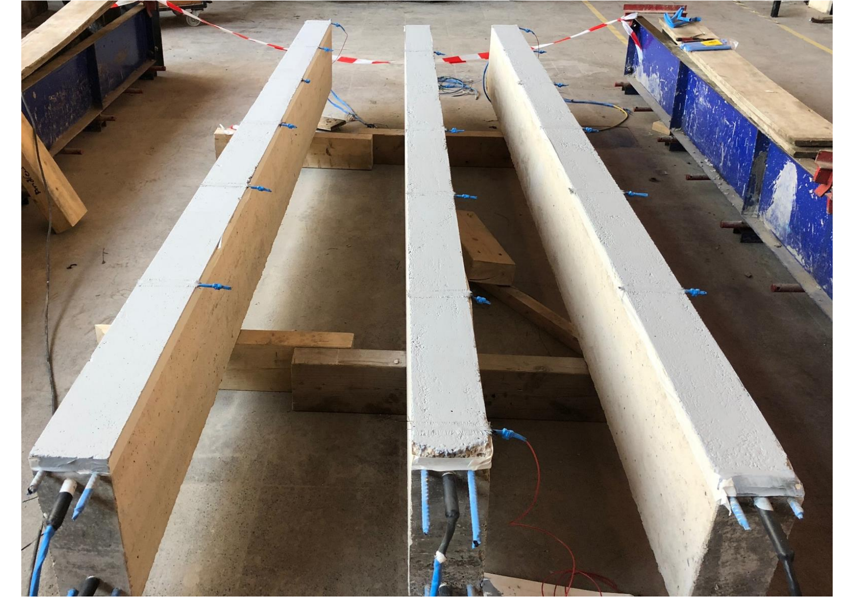
3m long beams coated with ZRP for polarization test
