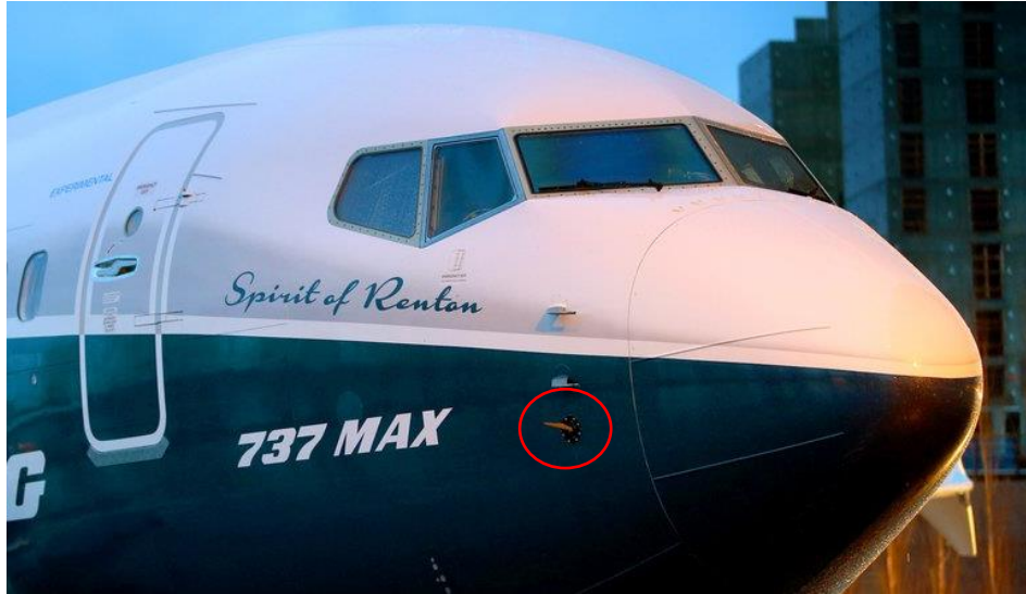
Figure 1. Boeing B737-800 Max nose mounted Angle of Attack vane [9]
