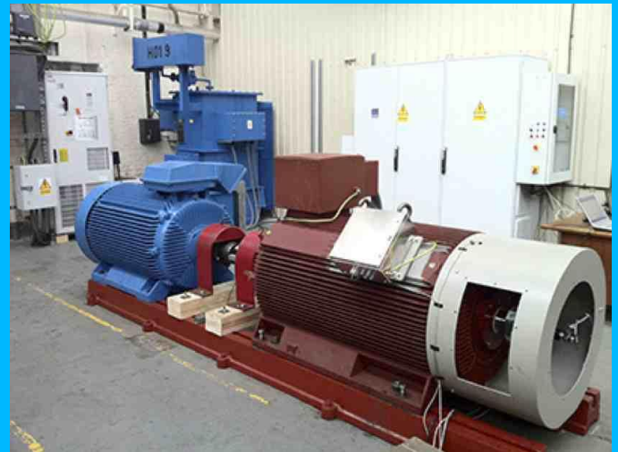
Fig. 1. 250 kW BDFM (front right) and the load machine on test rig.
