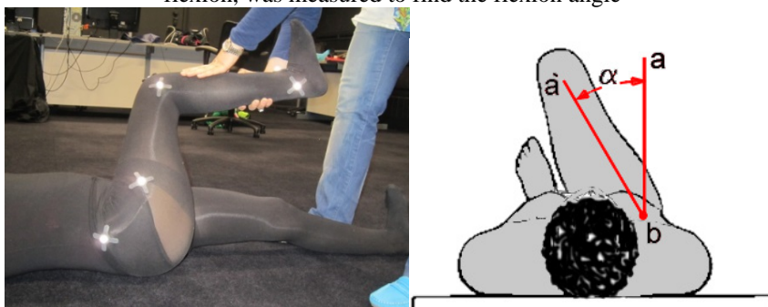
Fig. 4. To measure the adduction, the leg was positioned toward the centre of the body
