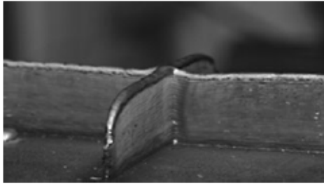
Figure 11 Deposition of cross structure(25)
