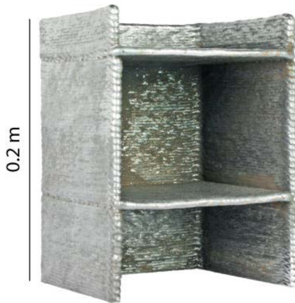
Figure 12 Horizontal features deposition without support(27)
