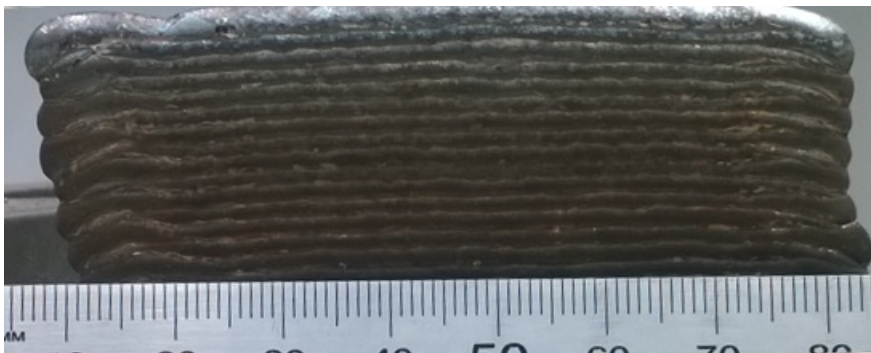
Figure 10 Single bead multi-layer WAAM part with controlled start and end
