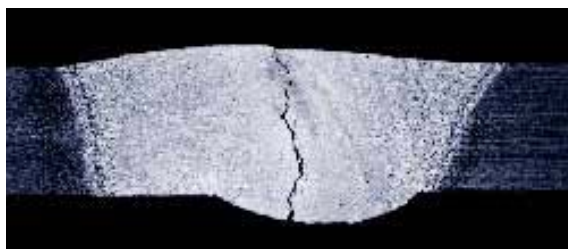
Figure 3 Solidification cracking in aluminium welding (93)
