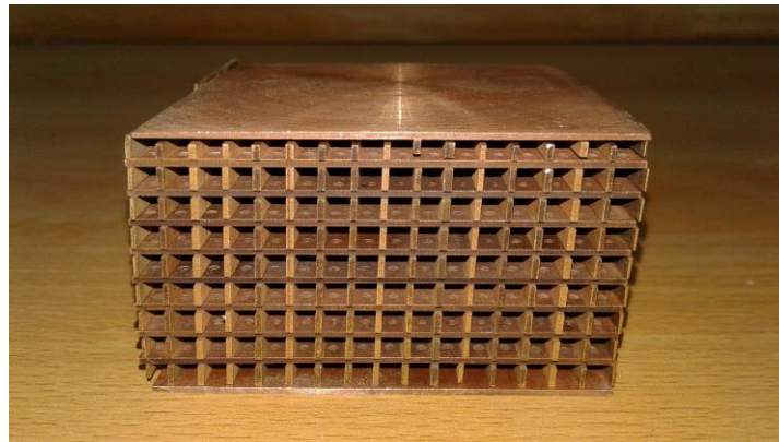
Fig. 6 Fabricated squarebore microhole3 (Cu) structure
