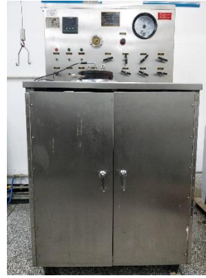
Fig. 2(b). Autoclave Curing device
