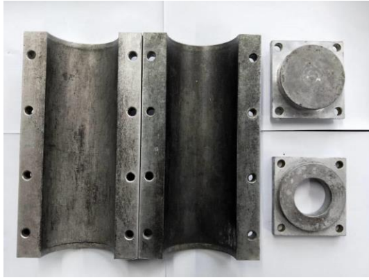
Fig. 2(a). Conservation mould of Cement sheath integrity
