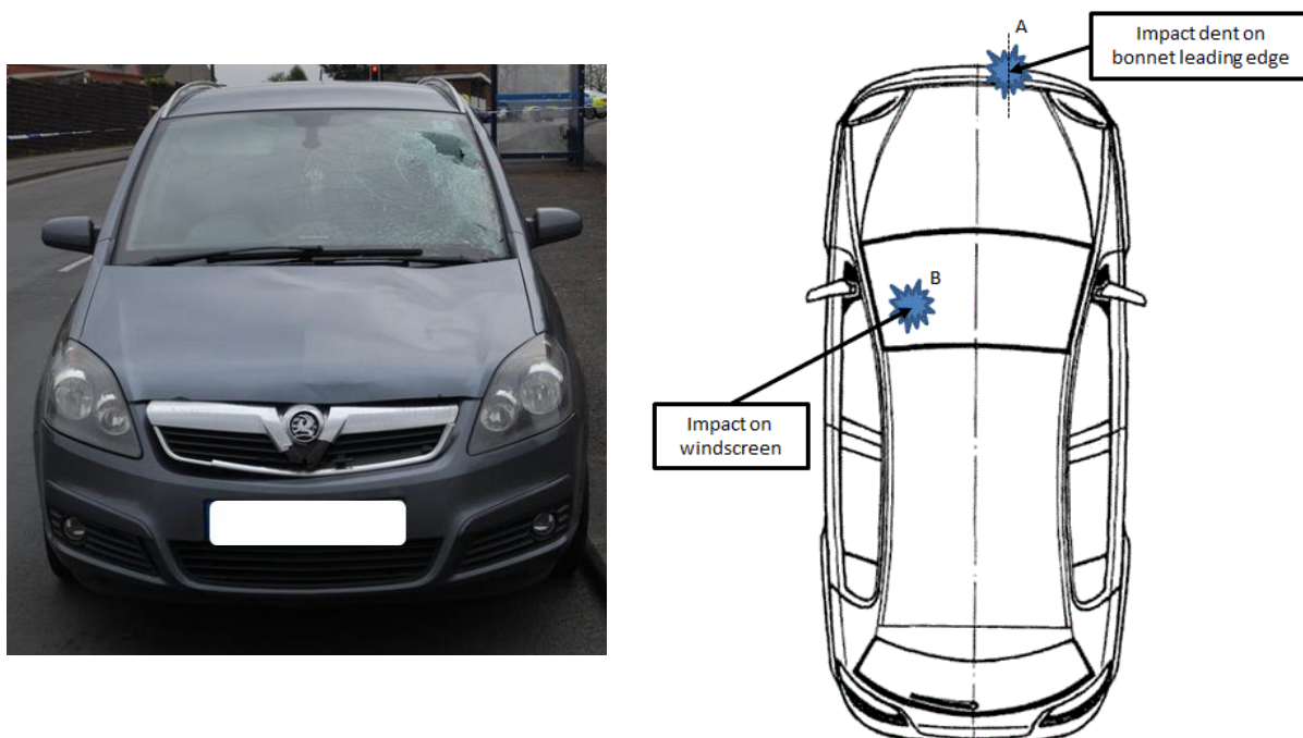
Figure 3: Evidence usually observed in car to pedestrian collision. (Real life accident, Left; Schematics, Right, W and H respective planar dimensions)
