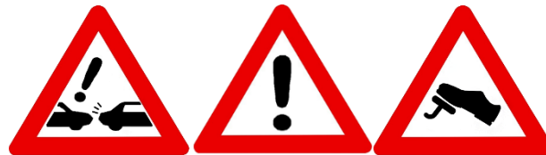
Fig. 3. Signs 1-3 for the Emergency Electronic Brake Lights (EEBL) feature
