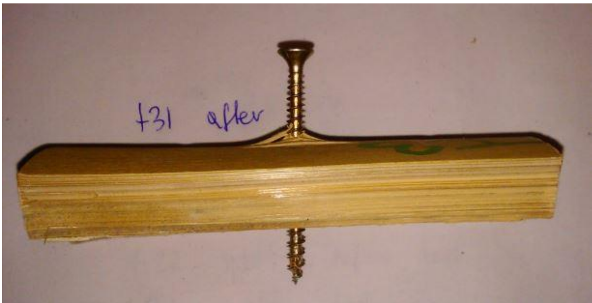
Figure 10: typical withdrawal failure mode
