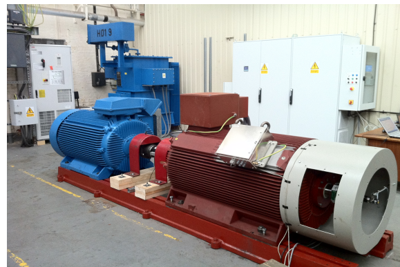
Figure 2: 250 kW BDFM (right front) on test bed
