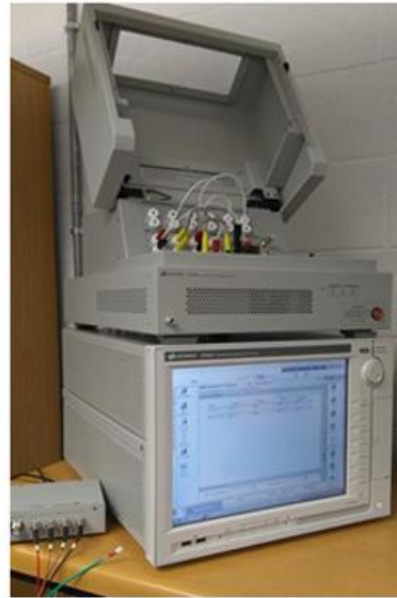
Fig. 1: (a) Graphical representation of the overall experimental setup, (b) The B1505A Power Device Analyzer, (c) Thermal chamber using resistive heating, (d) The thermal chamber connected to the temperature controller.
