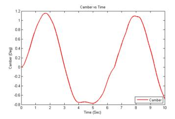
Fig. 17. Graph of camber vs time of adaptive system.
