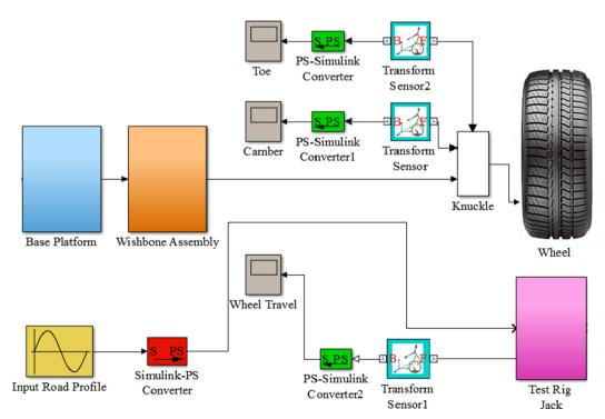
Fig. 5. Simulink block diagram of passive suspension system.
