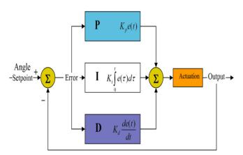
Fig. 7. Schematic of the PID control system.
