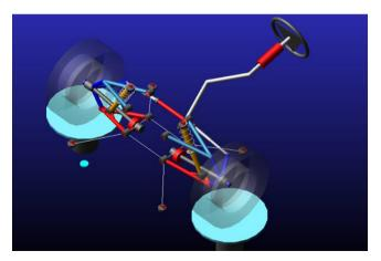
Fig. 9. SLA isometric view geometry model in ADAMS CAR.
