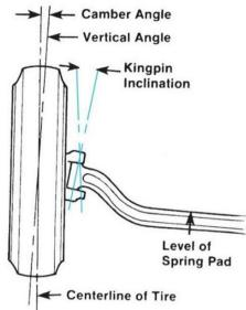
Fig. 1. Front suspension packaging.
