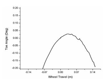
Fig. 21. Graph of toe vs wheel travel of passive system.
