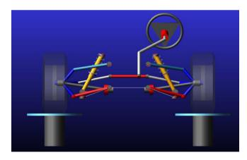
Fig. 8. SLA front view geometry model in ADAMS CAR.
