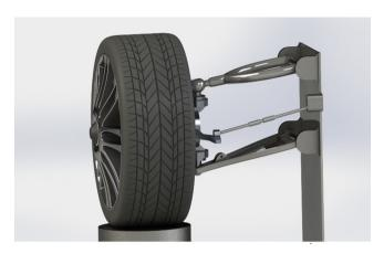
Fig. 4. SOLIDWORKS model of the setup with variable length upper arm and tie rod.
