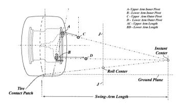
Fig. 2. SLA front view geometry.
