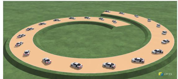
Fig. 15. Test (#4). Drift on clothoid. R_{ini} = 50m , R_{final} = 25m .
