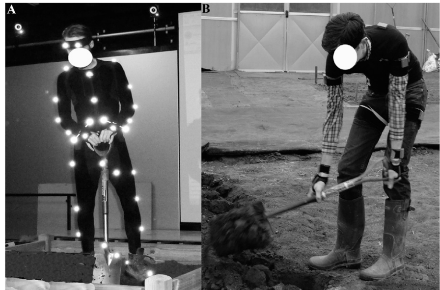
Fig. 1. Three-dimensional motion-capture systems used during digging trials [optical tracking (A), magneto-inertial (B)].
