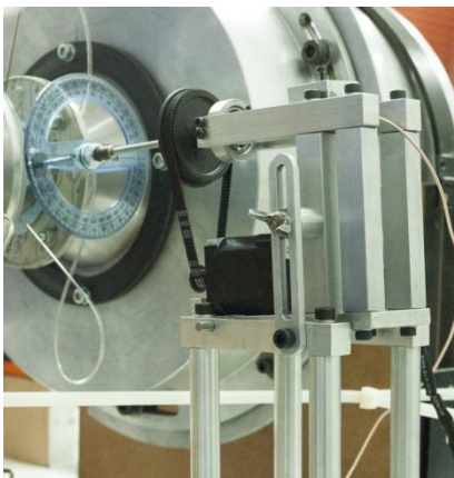
Figure 5. HWA probe positioning mechanism for angular and radial traverse of the HWA probe.
