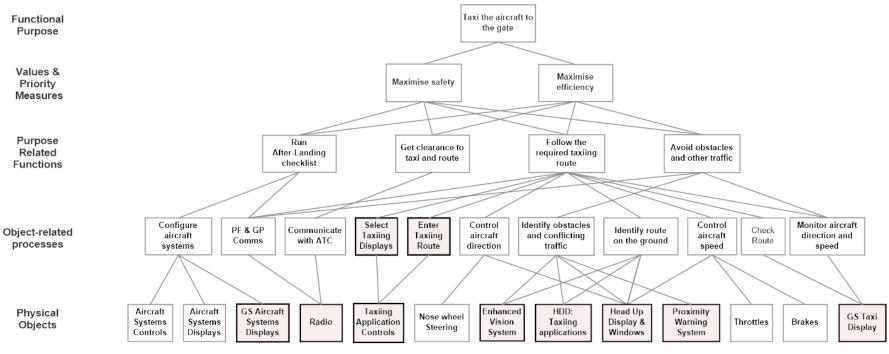
PF - Pilot flying, GP - Ground Pilot, GS - Ground Station
