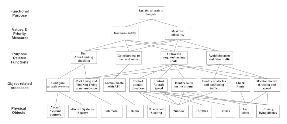
Fig 2 WDA abstraction hierarchy for taxiing the aircraft to the gate for two-pilot operations (baseline).
