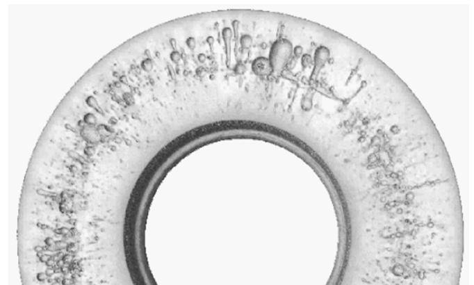
Fig. 4 Porosity in end ring: 3D reconstruction of the end ring 2D x-ray scan
