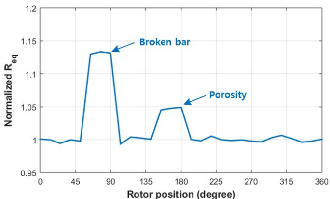
Fig. 9 3D FEA results of R_{eq} as a function of rotor position for broken bar and porosity located at 77 and 167 degrees (66 V, 50 Hz excitation)
