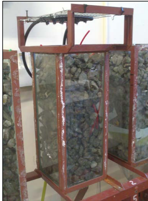
160 161 Fig. 1 Detail of the laboratory HFD model and the rainmaker.
