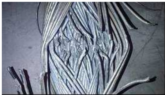
(a) Wire failure modes for V_i = 1328 m/s
