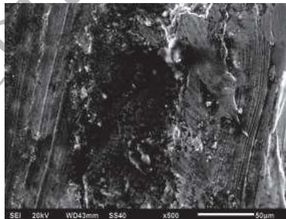
Fig. 13 Typical smearing of microstructure on impact on central region 2 of fractured wire for V_i = 1328 m/s (SEM 500 x mag.)
