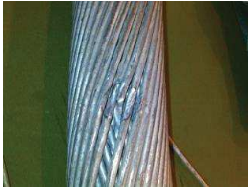
(f) V_i = 297 m/s - Fragment penetration depth = 0mm (0 layers of wires)
