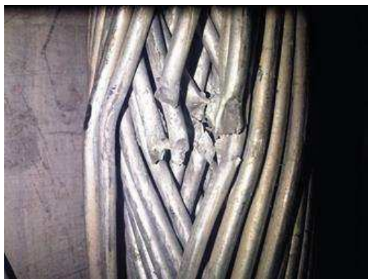
(c) Wire failure modes for V_i = 501 m/s
