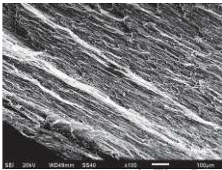
(b) Base region: V_i = 680 m/s (SEM 100 x mag.)
