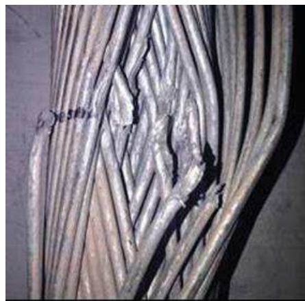
(b) Wire failure modes for V_i = 680 m/s
