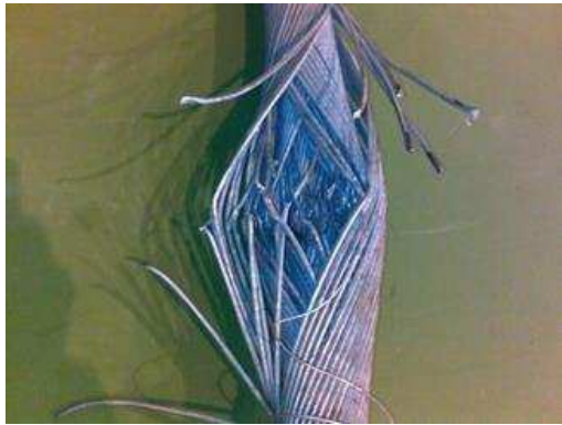
(a) V_i = 1328 m/s - Fragment penetration depth = 25mm (5 layers of wires)
