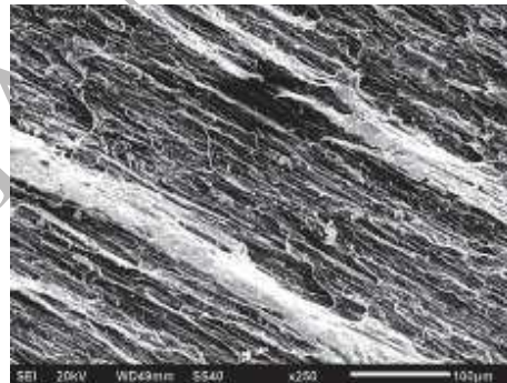
(c) Base region: V_i = 680 m/s (SEM 250 x mag.)
