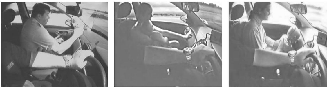
Figure 2: Pictures of passengers bracing when subjected to pre-braking [4]
