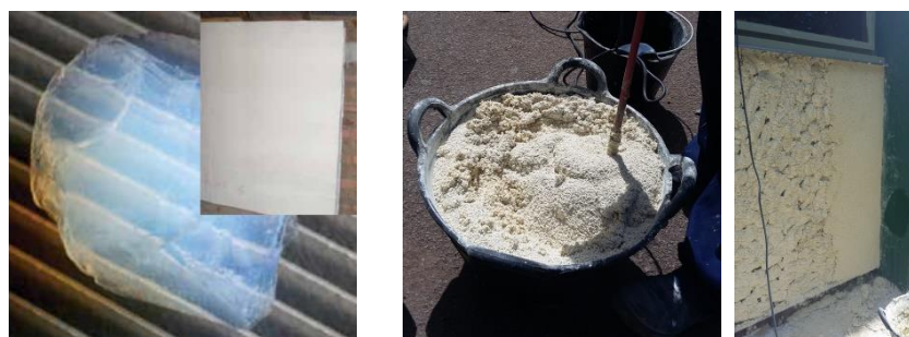
Figure 7. Image of aerogel and aerogel mortar insulation
