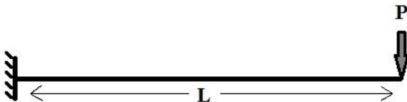
Figure 3. The configuration of a cantilever straight beam
