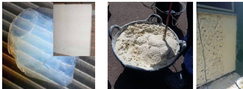
Figure 2. Image of aerogel and aerogel mortar insulation
