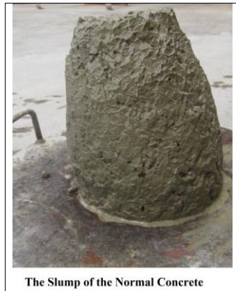
The Slump of the Normal Concrete Figure 6: Slump of the normal concrete
