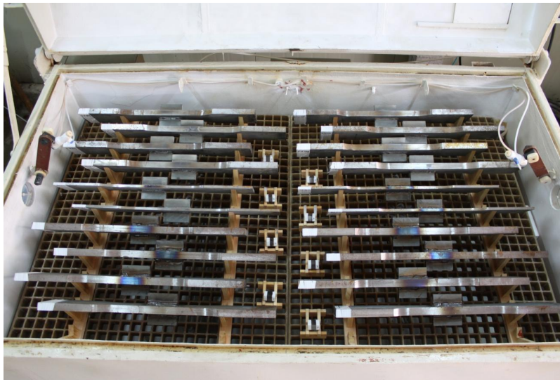
Figure 2: Salt bath used for corrosion exposure. A number of specimens were placed in a single test chamber and were rotated from time to time to ensure uniform exposure to salt spray
