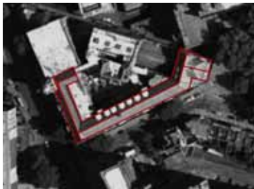
Figure 4: roof edge detection final results using method/algorithms
