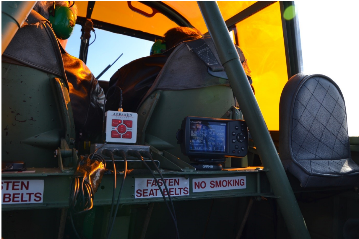
Figure 5, Flight Test Data Acquisition System Installation (AHRS/GPS 2)
