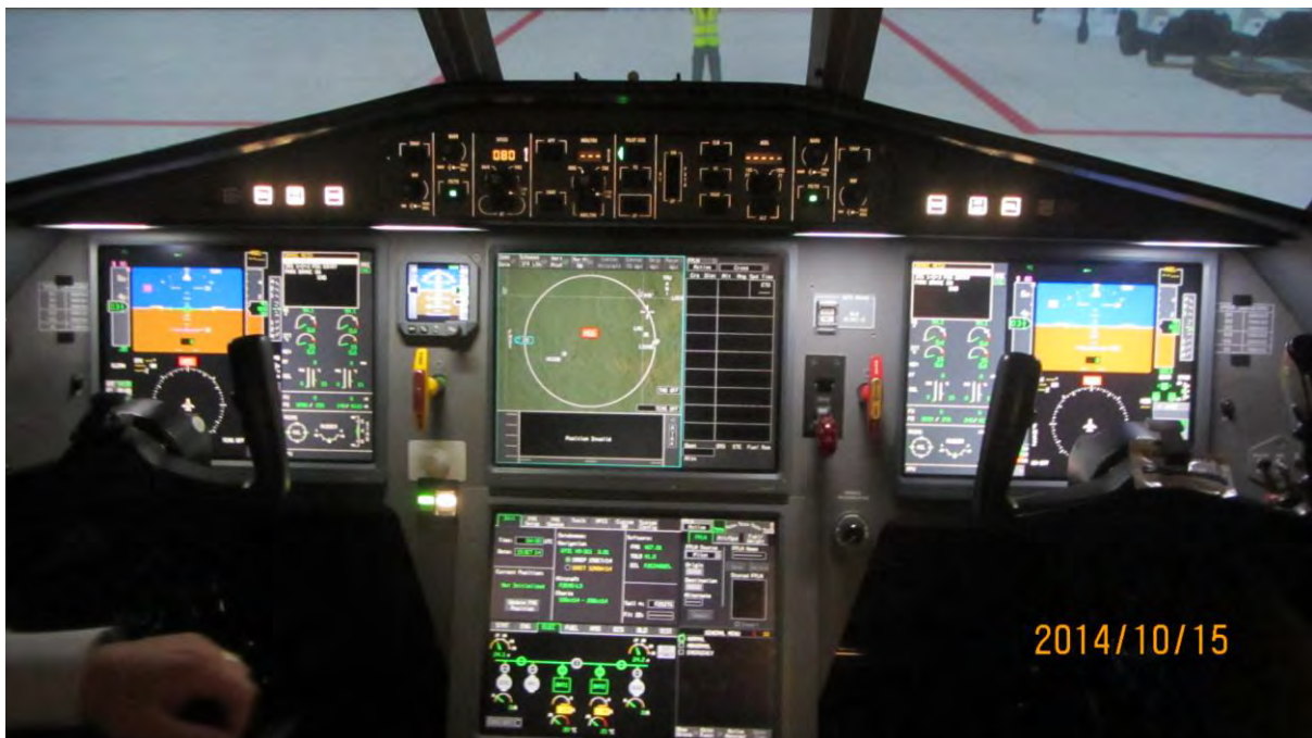
Figure 10, G450/550 Full Flight Simulator with Honeywell Primus Avionics/FMS
