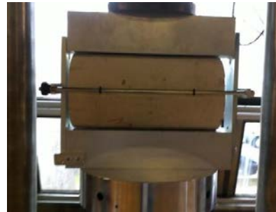
Fig. 7: Splitting test on cylindrical specimen
