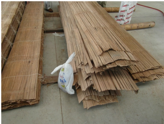
Figure 6: Esterilla (Colombia) or caña picada (Ecuador): Sheets of bamboo formed by physically opening / splitting a large diameter culm along its length and then unrolling it (Kaminski, 2016)
