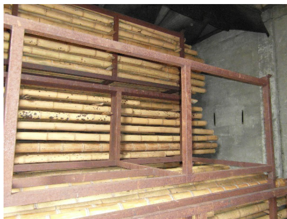
Figure 45: Kiln drying of bamboo, Colombia (Kaminski, 2016)
