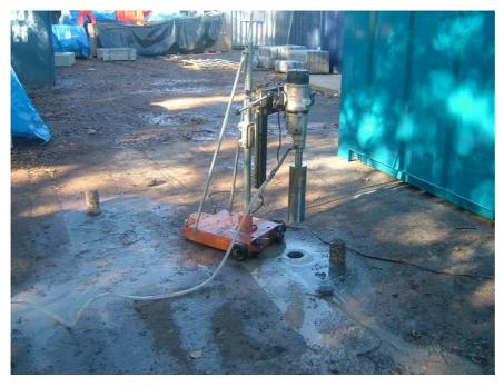
Figure 134 Core sample taken from middle and end part of the trial car park at the Lowdham Grange site
