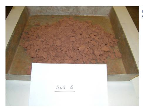
Figure 19 Silty sand soil (Soil B)
