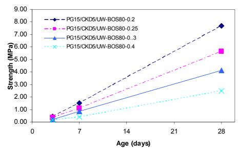
The mix with an L/S ratio of 0.2 achieved the highest strength at a test age of 28 days regardless of the weathering condition of the slag (Figures 26 and 27). The results also indicate that PG15/CKD5/BOS80-0.2 gains strength at a higher rate compared with other mixes.
