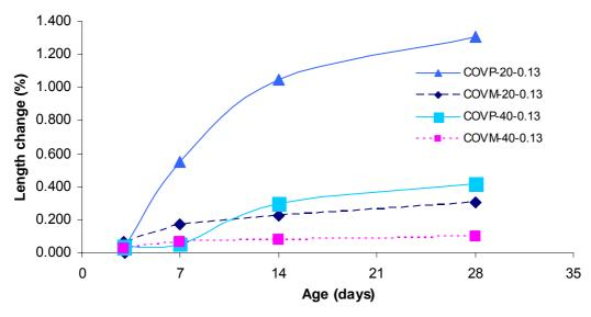
Figure 88 Effect of temperature on length change of paste and mortar mixes
