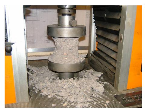
Figure B14 A concrete sample after crushing
