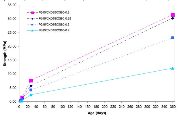
Figure 60 Long-term compressive strength development of PG-CKD-BOS paste mixtures (50 mm cubes)
