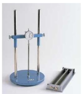
Figure 86 Apparatus for determination of length change
