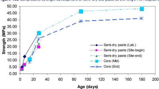
Figure 132 Compressive strength development of semi-dry site paste at the King's Mill Hospital site
