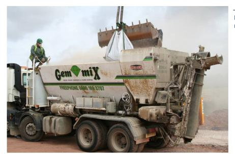
Figure 121 Loading the mixer with blended powder
