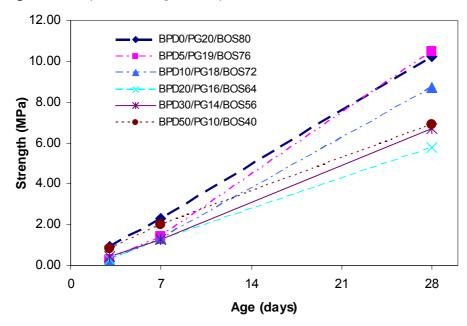
The effect of the amount of PG and BPD on binary and ternary combinations of PG-BOS and BPD-PG-BOS at different ages is shown in Figures 36 and 37 respectively. Figure 35 indicates the optimum percentage for PG in the binary combination is 20% and shows a dramatic decrease in strength when PG is increased from 20% to 60%.
