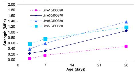
Figure 50 Compressive strength development of lime-BOS mixtures
