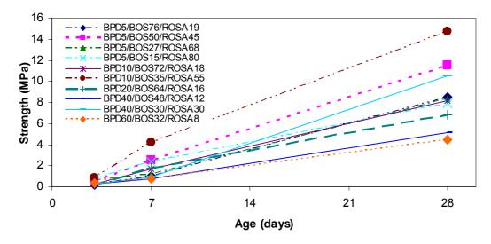
Figure 47 Compressive strength development of ROSA-BOS-BPD mixtures
