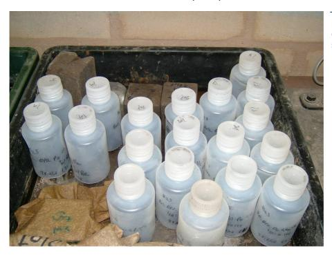
Figure 68 Plastic bottles containing paste specimens for H<sub>2</sub>S check
