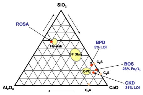
The composition of BOS is quite different from that of BF slag (GGBS). This is due to the nature of the process from which these materials are derived. GGBS is produced during the production of steel in the blast furnace while BOS is obtained from basic oxygen furnace process. Figure 17 presents a general schematic that depicts the blast furnace feedstocks and the production of blast furnace co-products (iron and slag).
