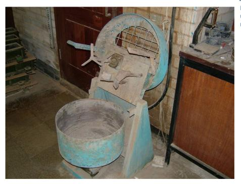
**Figure B2** Pan mixer used to make concrete mixes
