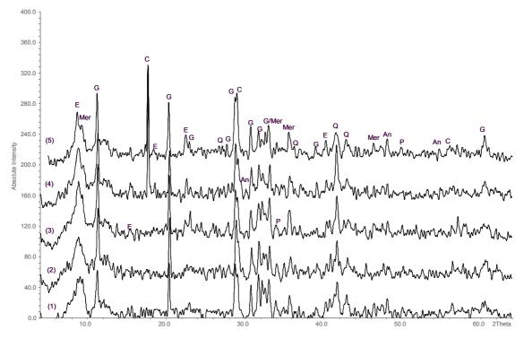
The phases related to slag (merwinite) were identified within the matrix, indicating the presence of unhydrated slag particles within the mixture (Figure 80). As the slag is a slow-reacting material, it may be that only a low percentage of the total slag fraction reacts at 28 and even 180 days.
