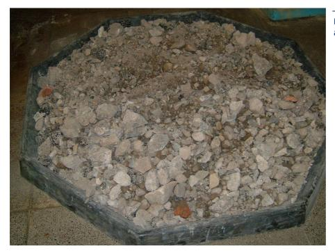
Figure 12 Recycled aggregate used
