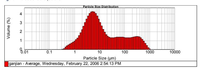
Figure 8 Particle size analysis of BPD
