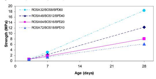
Figure 48 Compressive strength development of BOS-ROSA-BPD mixtures
