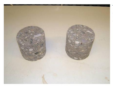
Figure 135 RCC core samples taken from different locations of the trial car park at the Lowdham Grange site
