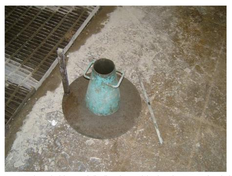
**Figure B4** Slump test truncate cone and base
