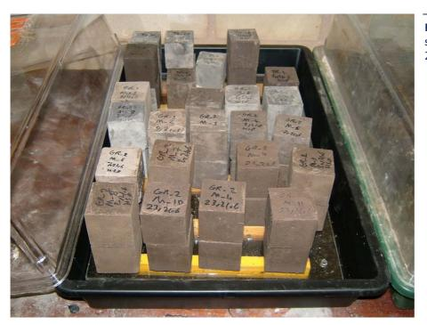
Figure B8 Paste samples stored in a container at 20±2° C and 98% RH
