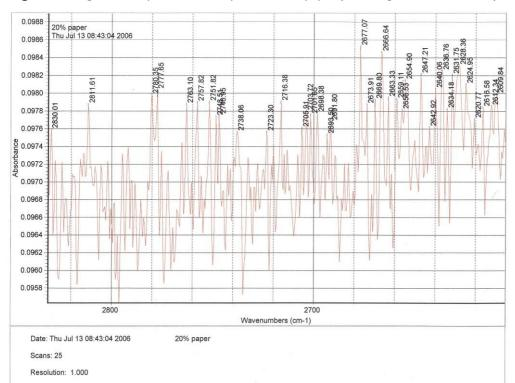
Figure 73 Magnified IR spectrum of sample with 20% paper (wavelength 2600-2800 cm<sup>-1</sup>)
