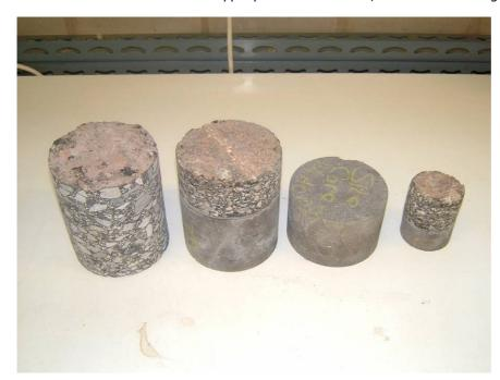
Figure 131 Core samples taken from different locations in the trial road at the King's Mill Hospital site
