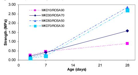
Figure 55 used data from Tables 34 and 35 to present a comparison of binary mixtures of BPD-ROSA with the lime/MKD-ROSA mixtures. The mixture incorporating BPD achieved much a higher compressive strength compared with those made with hydrated lime and MKD. This result is similar to those achieved with binary combinations of BPD-BOS. As mentioned previously, this could be due to cementitious compounds present in BPD resulting in formation of more cementitious matrix within 28 days.
