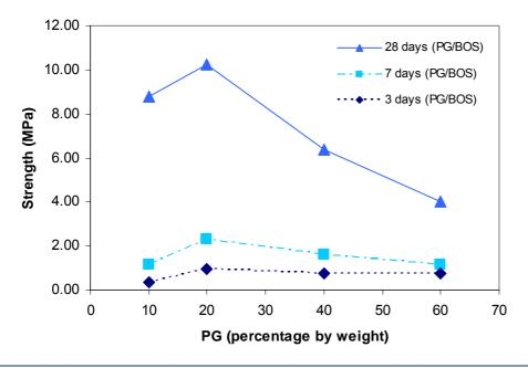
Figure 37 Compressive strength of BPD-PG-BOS mixes versus BPD content
