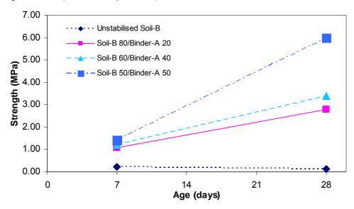
Binder-A (Coventry Binder) performed relatively better with Soil-B (Figure 63) than with Soil-A (Figure 64). Soil-A was taken from one of the trial sites (see section 4.3) long before the trial was due to begin out. But this soil was not available later and another source of soil (Soil-B) was provided from the same site for the site trial tests.
