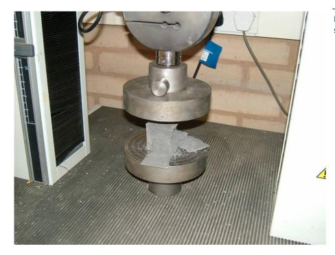
Figure B12 A paste sample after crushing
