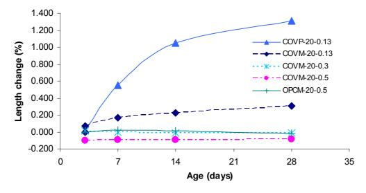
Incorporating aggregate in the mixture resulted in less expansion, mainly because less binder was used in the mix and the constraining effect of fine and coarse aggregate in the system. The expansion of mortar samples made with a similar water to binder ratio was only about 15% of that of the semi-dry paste. In addition, the lower L/S ratio led to greater expansion in the mortar samples.
