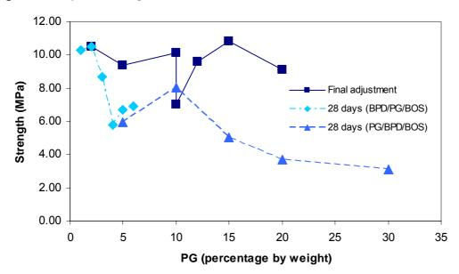
Figure 42 Compressive strength of various combinations of PG, BPD and BOS versus content
