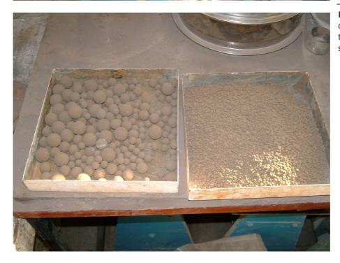
**Figure B6** Metallic balls of different sizes used in the ball mill to grind the slag
