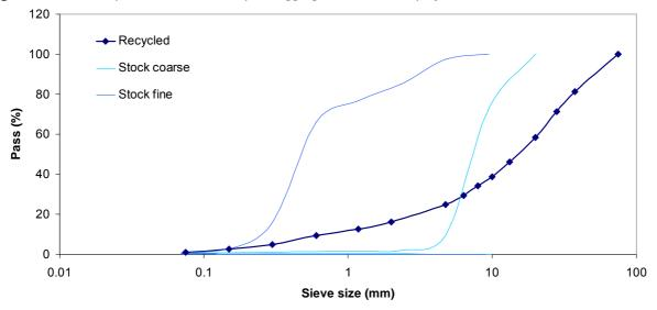
As shown in Figure 14, the calculated coarse and fine fractions of the recycled aggregate complied with the requirements of BS-EN 12620-2002.
