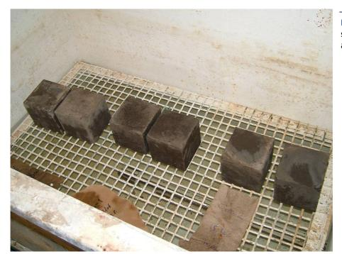
Figure B9 Concrete samples stored in a tank at 20±2° C and 98% RH
