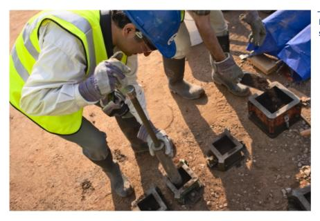
Figure 119 Sampling the stabilised soil
