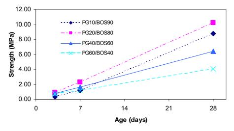
Figure 35 Compressive strength development of BPD-PG-BOS mixes
