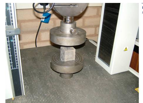
**Figure B11** A paste sample before crushing
