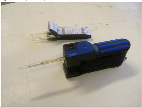
Paste samples containing 5, 10, 15, 20 and 50% extra paper was tested at 1, 14 and 28 days curing (Figure 76). No change in colour was observed during testing of different samples (Figure 77). This indicated the absence of hydrogen sulphide in the airtight containers and confirmed that hydrogen sulphide was not formed even when the binder contained a large amount of paper (50%).
