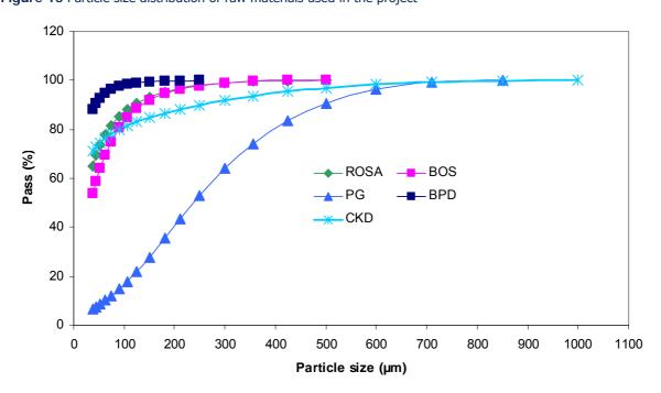
Figure 15 Particle size distribution of raw materials used in the project
