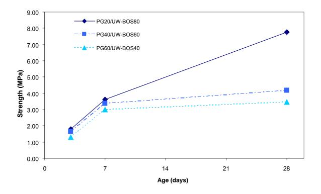
Figure 22 Compressive strength development of pastes containing CKD, PG and BOS
