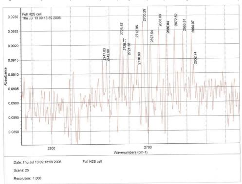
Figure 71 Magnified IR spectrum of pure hydrogen sulphide (wavelength 2600–2800 cm<sup>-1</sup>)
