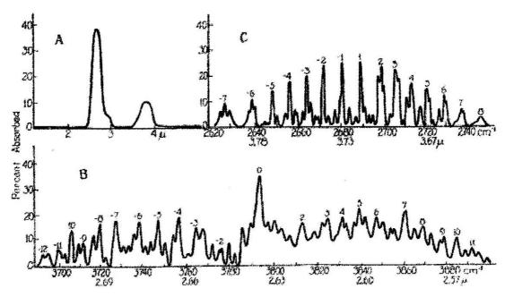
Figure 70 shows the IR spectra of the gas extracted from specimens containing 10 and 20% paper. No distinctive difference can be seen between the spectrum obtained with an empty cell and the one containing extracted gas.
