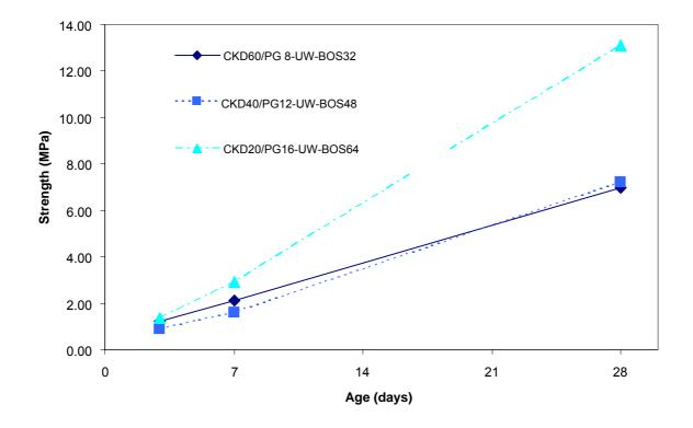
Figure 23 Compressive strength versus CKD content
