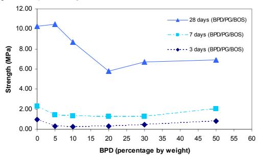
The role of PG in both binary and ternary systems is shown in Figure 38. In the ternary system, increasing the PG content up to 16% in the mix resulted in a reduction in compressive strength. However, a further increase in the amount of PG led to a considerable improvement in strength, with the maximum value of 10.5 MPa as the optimum in this particular combination (Table 24).
