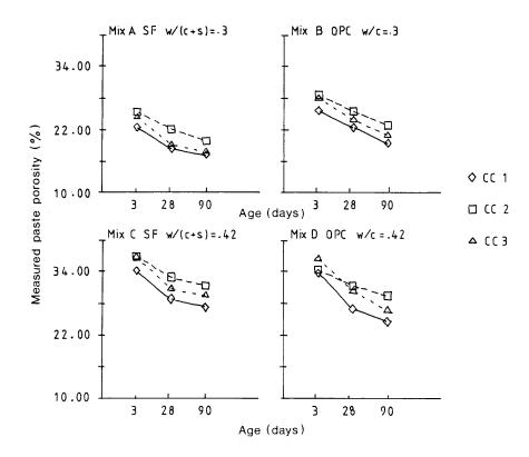
Figure 8. Porosity results for paste samples (obtained by helium intrusion).
