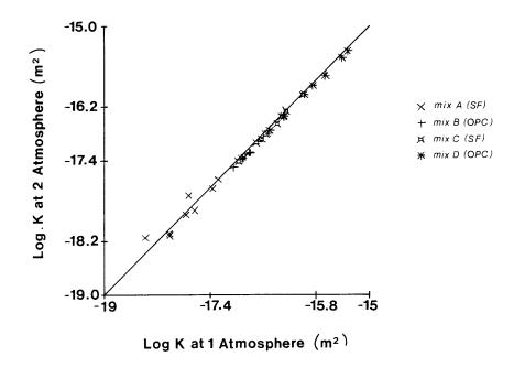
Figure 2. Relationship between measurements of the oxygen permeability K made at 1 atmosphere pressure drop and those at 2 atmospheres. The line drawn is that of equality (Y=X).
