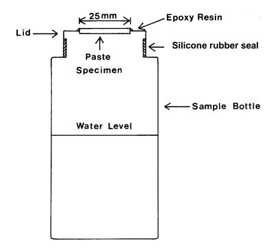
Figure 4a. Detail of bottle for vapour transmission measurement.
