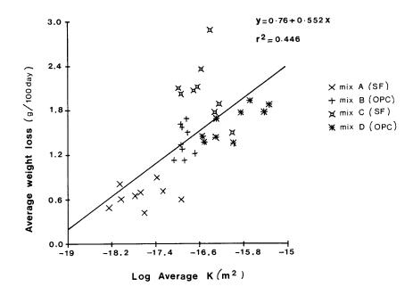
Figure 9. Relationship between the permeabilities to oxygen and water.
