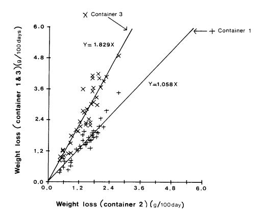
Figure 6. Relationship between the weight losses of equivalent samples in the different containers.
