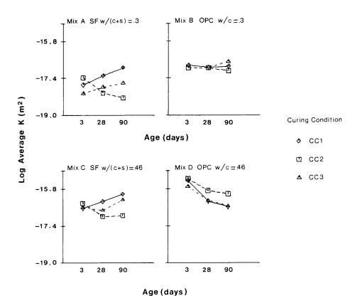
Figure 3. Oxygen permeability K calculated from an average of the readings at 1 and 2 atmospheres.
