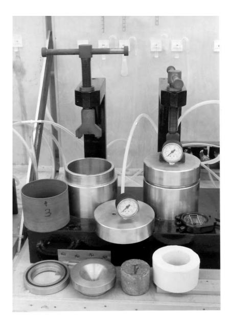
Figure 1. Leeds Gas Permeameter.
