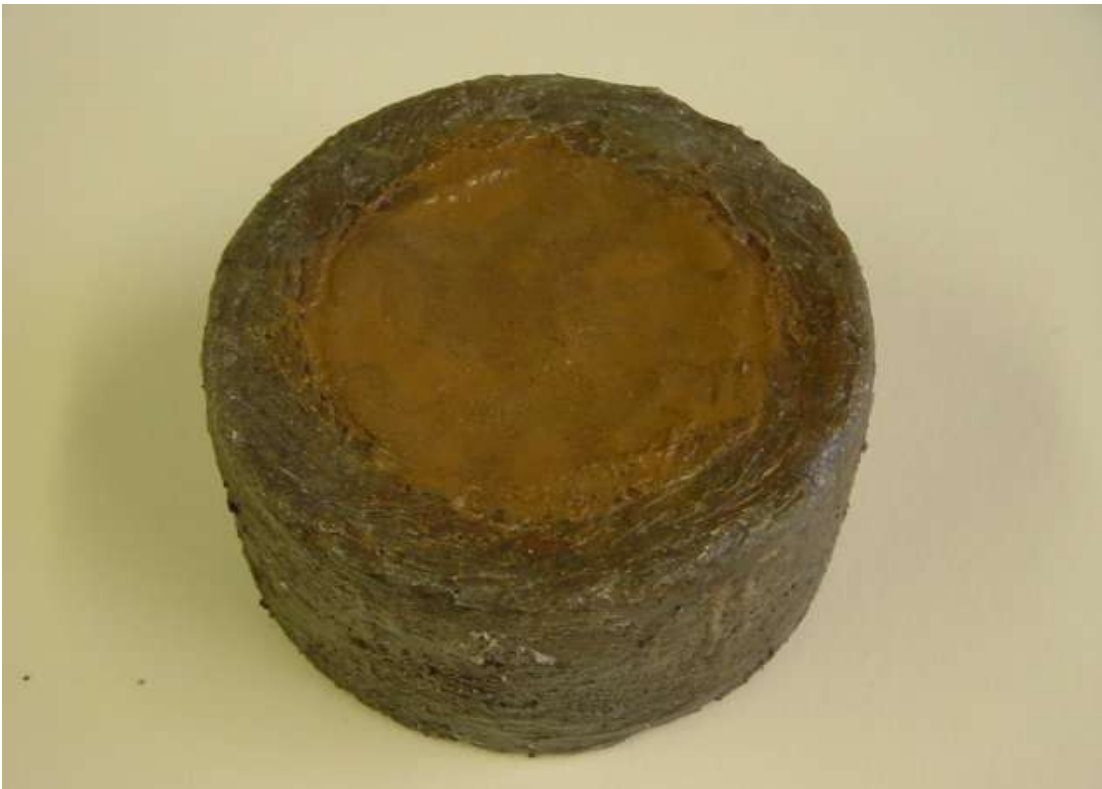
Fig. 4.11: The set up of bottom layer mix and compacted clay with silicone rubber round the rim and inside wall to prevent ingress of leachate from rim and interfaces.
