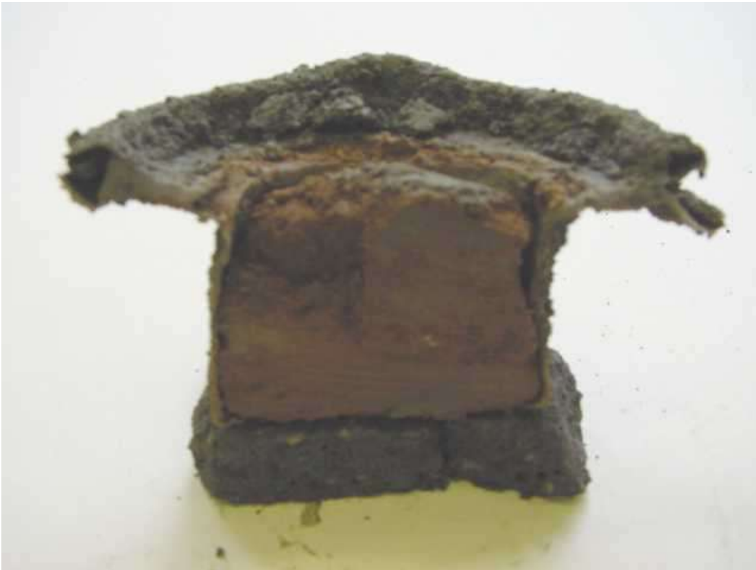
Fig. 4.14: Cut through the dismantled multi layer sample.
