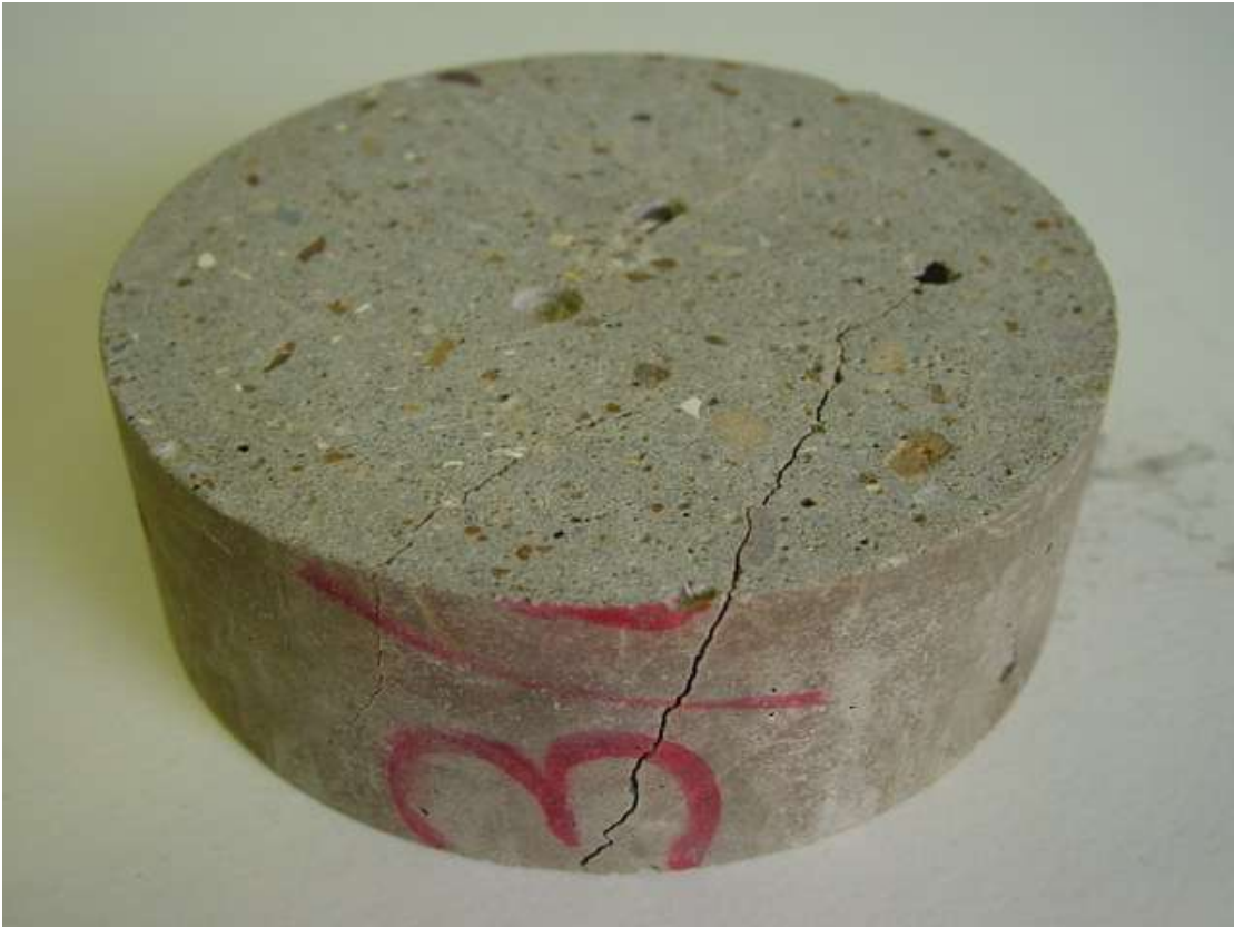
Fig. 4.9: Narrow cracks induced in the F.R. mortar disc.
