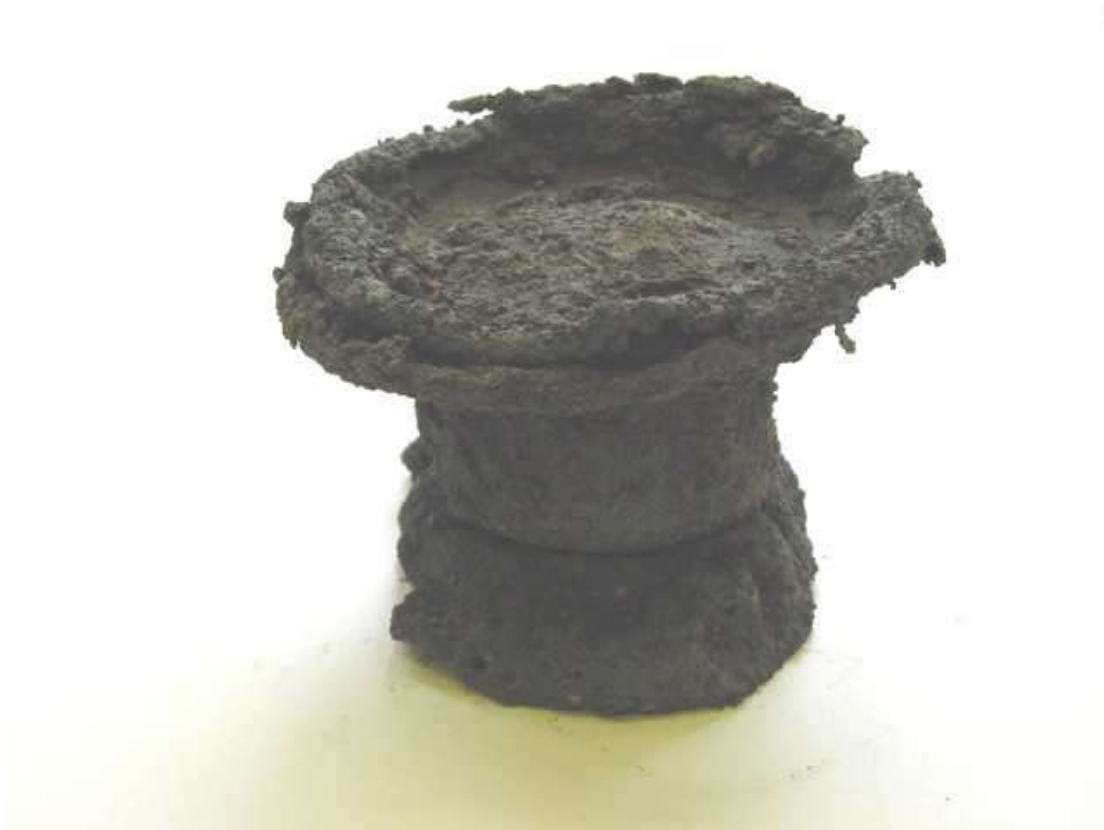
Fig. 4.13: Multi layer sample after taken out of the test rig.
