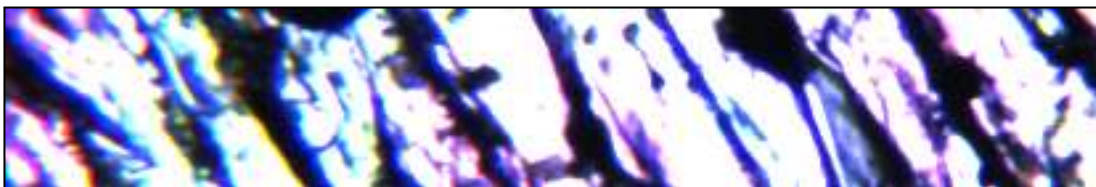
Figure 2.24 Chrome alumina slag in optical thin section showing characteristic purple body colour from \text{Cr}^{3+} in solution in the alumina matrix. Image width is 120 \mu\text{m}
