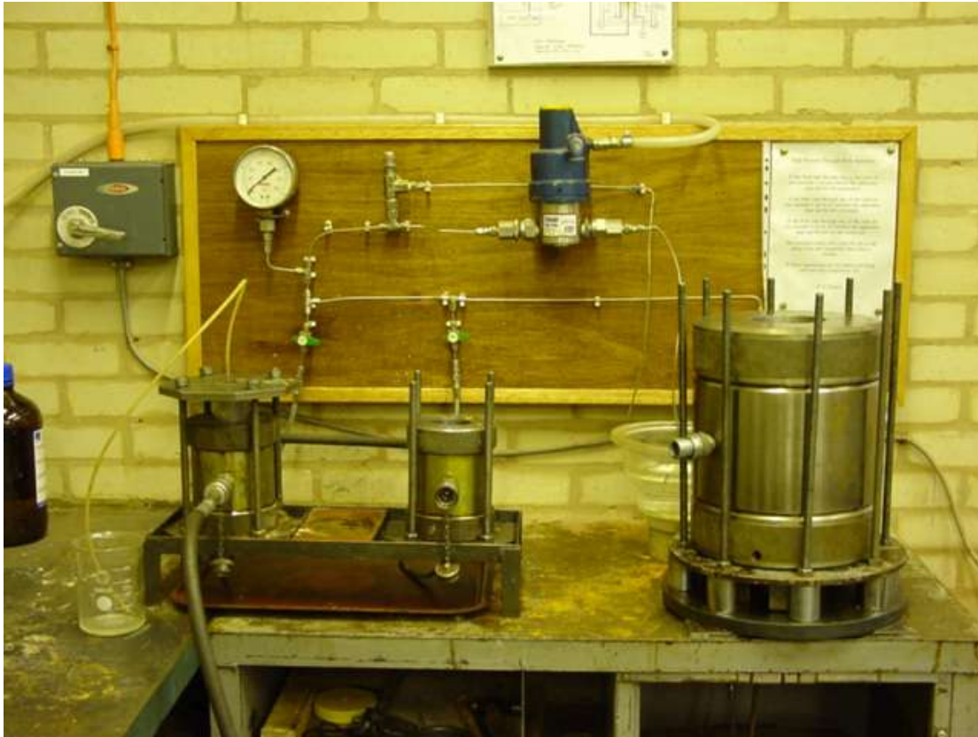
Figure 4.2: High-pressure apparatus at Coventry, showing two small cells (for 54 mm diameter samples) and one big cell (for 100 mm diameter samples) together with liquid pump and pressure gauge.
