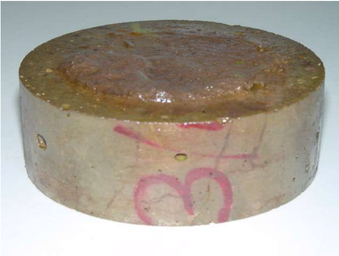
Fig. 4.10: Cracked sample after clay has sealed the cracks.
