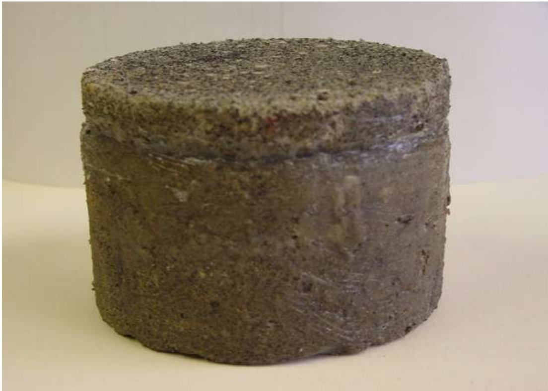
Fig. 4.12: Multi layer sample with partially compacted clay inside it.
