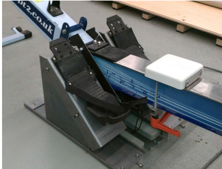
Fig 1: Footplates cantilevered from floor mounted force plates.
