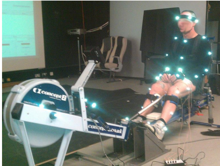
Fig 2: Subject with retro-reflective markers attached for motion capture.
