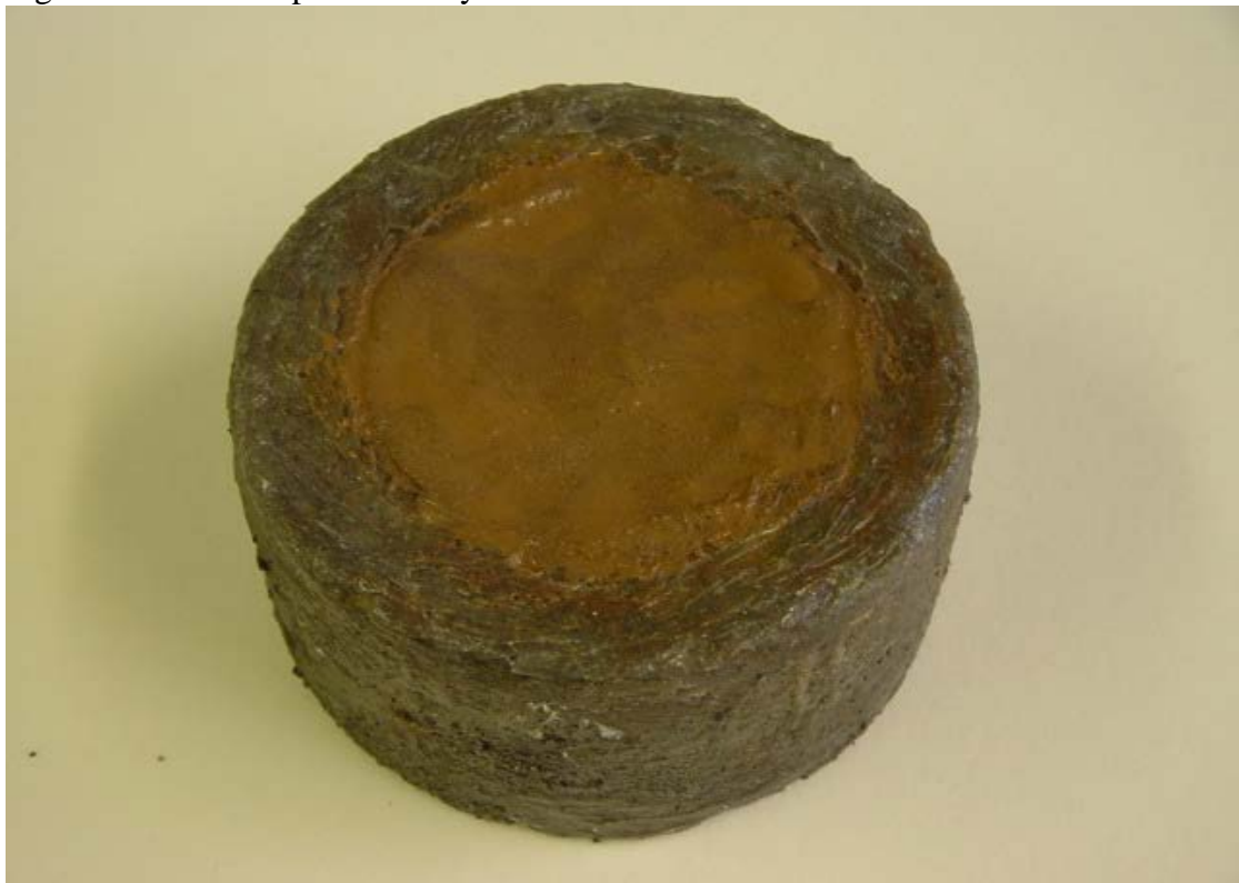
Fig. 7: The set up of bottom layer mix and compacted clay with silicone rubber round the rim and inside wall to prevent ingress of leachate from rim and interfaces.
