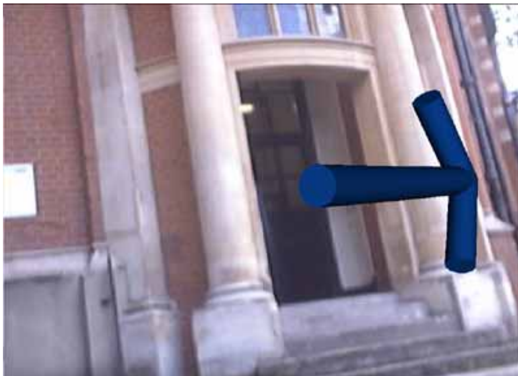
Figure 3 Augmented reality representation: a computer vision sensor recognises the doorway outline, and augments the video stream with virtual information (the direction arrow). Developed as part of the LOCUS project
