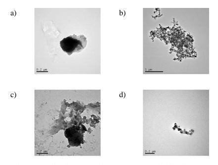
Figure 1. TEM micrographs of PM for 303 CAD bTDC: a) Near-spherical droplets b) Large agglomerates c) wet diesel like-particle and d) diesel-like particles
