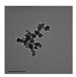
Figure 2. TEM micrographs for advanced injection timing settings.
