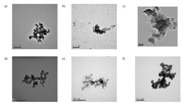
Figure 3. Example of micrographs for the different condition studied: 303 CAD bTDC a) noEGR b) EGR c) REGR, 335 CAD bTDC d) noEGR e) EGR and f) REGR.
