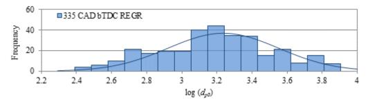
Figure 5. Primary particle size distribution for 335 CAD bTDC at noEGR, EGR and REGR.
