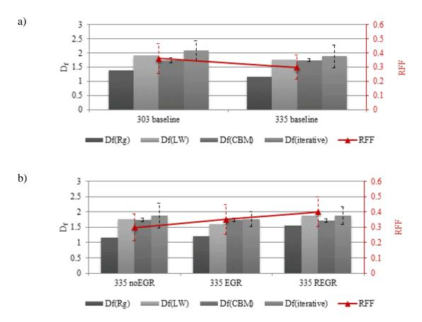
Figure 9. Fractal dimension calculated using different methods: a) Baseline comparison and b) 335 CAD bTDC injection timing noEGR, EGR and REGR
