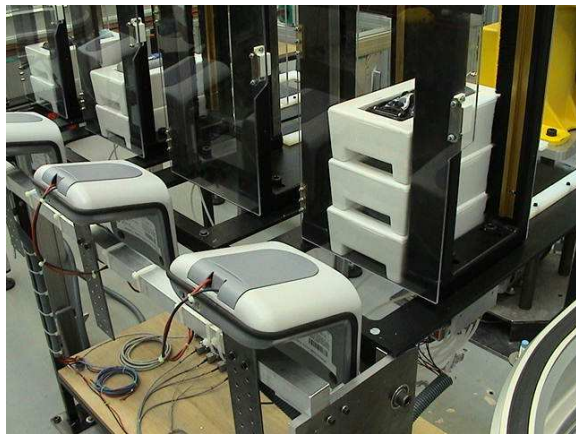
Fig. 8. Work in process buffer for packing robot.
