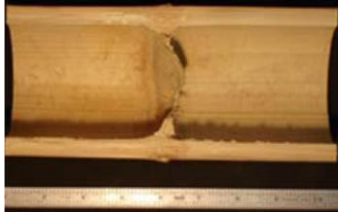
a) longitudinal section of bamboo culm showing portions of internodes to either side of node
