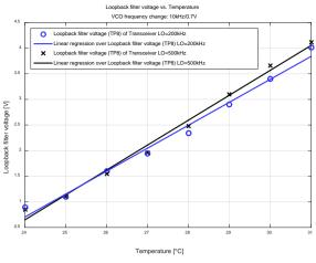
Fig. 6. Temperature dependency of the system
