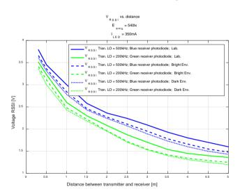
Fig. 7. Received signal strength in different distance
