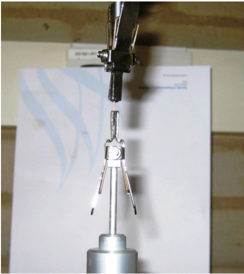
Figure 3- measuring the tensile strength of fibres using Fine Wire Grip
