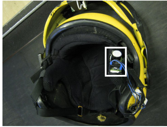
Figure 3: CO 2 sensor positioning within the EOD suit helmet.
