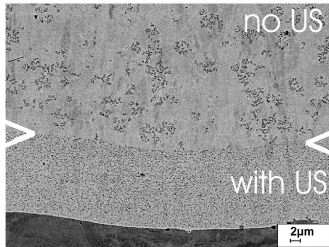
Figure 4. Well-dispersed \text{TiO}_2 particles under ultrasound conditions (lower part from substrate up to the markers >< ) and nano-particle agglomeration under silent conditions (upper part) in a Ni coating. Adapted from Ref. [44], with permission from Elsevier.
